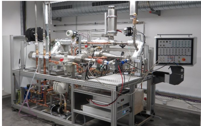
Pankl Turbosystems test stand for electric compressors
